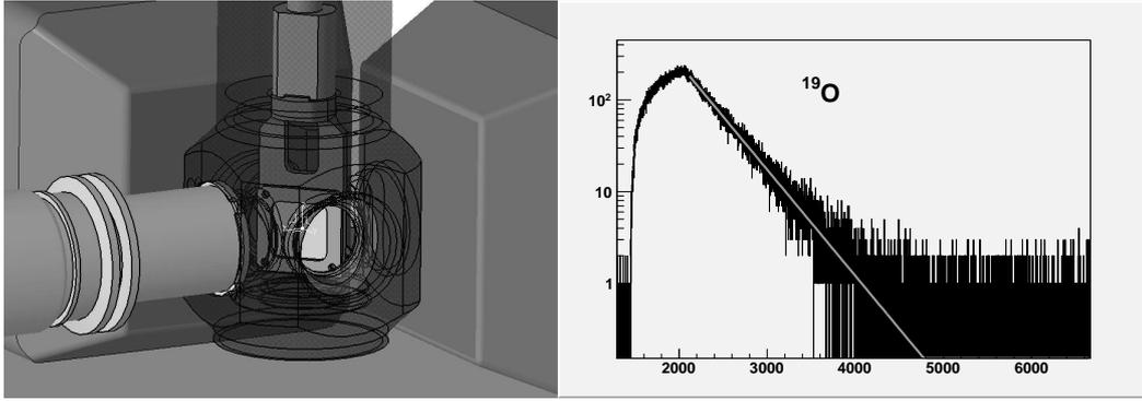
**FIGURE 1.** Left: Drawing of the experimental setup used to study the electron screening effect. The target is located inside a cryostat and surrounded by two EXOGAM germanium clover detectors, one plastic and one LaBr3 scintillator (not shown here) placed in a close geometry. Right: A single implantation and decay curve (counts versus time in seconds) measured for  $^{19}\text{O}$  using the plastic scintillator [12].
