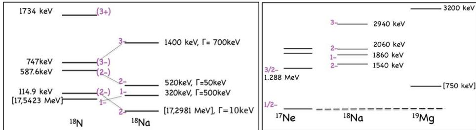
Fig. 2. Left: Level schemes for  $^{18}\text{Na}$  as found from the Anar $\chi$  fit and for  $^{18}\text{N}$ , its mirror nucleus. Right : Level scheme for two-protons radioactivity of  $^{19}\text{Mg}$ .
