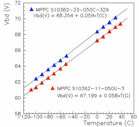
Fig. 2. The  $V_{BD}$  vs  $T$  for the MPPC of  $1 \times 1 \text{ mm}^2$  and  $3 \times 3 \text{ mm}^2$
