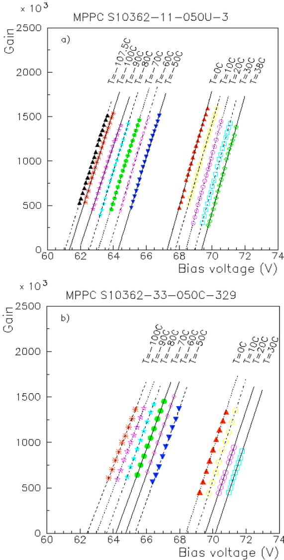
Fig. 1. The  $G$  vs  $V_{bias}$  for the MPPC of  $1 \times 1 \text{ mm}^2$  (a) and  $3 \times 3 \text{ mm}^2$  (b) at different temperatures.
