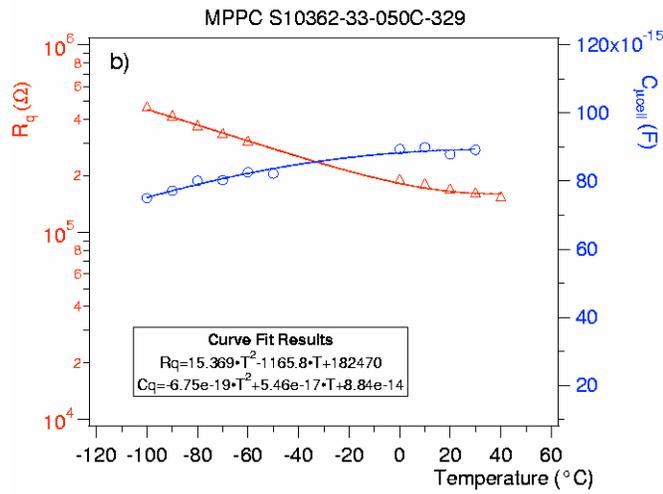
Fig. 4. The  $R_q$  vs  $C_{\mu\text{cell}}$  as a function of  $T$  for the MPPC of  $1 \times 1 \text{ mm}^2$  (a) and  $3 \times 3 \text{ mm}^2$  (b).
