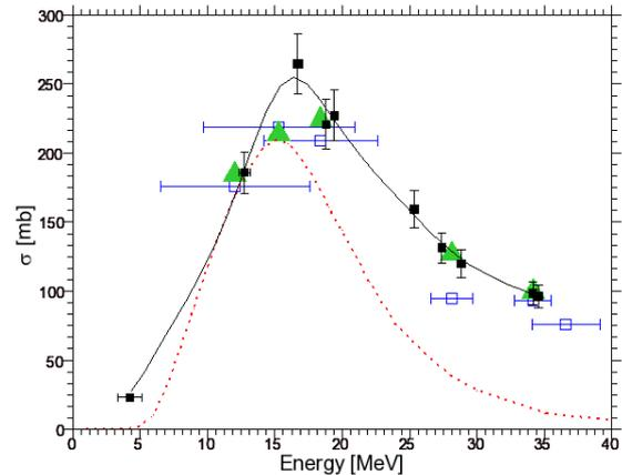
**Fig. 8.** Excitation function for the  $^{27}\text{Al}(^3\text{He}, 2p)^{28}\text{Al}$  beam monitor reaction; ■: our data. □: Frantsvog *et al.*, ▲: our data averaged on the same energy spread for comparison with the ones of Frantsvog *et al.*. Dashed line: TENDL-09 data base. Solid line: a eye guide of our data.
