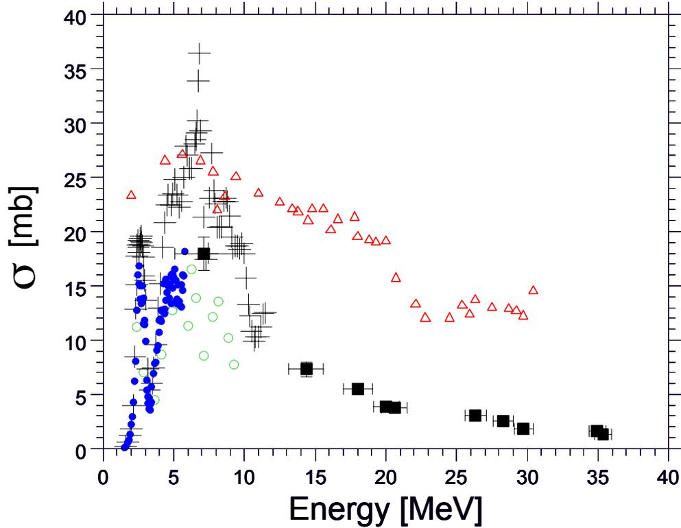
**Fig. 4.** Excitation functions for the  $^{12}\text{C}(^3\text{He},n)^{14}\text{O}$  reaction. ■: our data. ○: Hahn and Ricci. †: Osgood *et al.*. △: Singh. ●: Cirilov *et al.* modified by NNDC [21]
