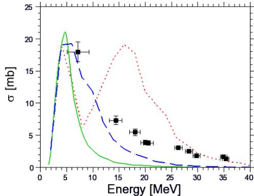
**Fig. 5.** Excitation functions for the  $^{12}\text{C}(^3\text{He},n)^{14}\text{O}$  reaction. ■: our data. Dotted line: TENDL-09 data base calculated with TALYS using default parameters. Solid line: population of the  $^{14}\text{O}$  ground state only, calculated with TALYS and default parameters. Long dashed line: the same but calculated with larger number of discrete states considered in all nuclei.
