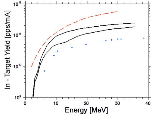
**Fig. 6.** Comparison of the thick target production yields for the  $^{12}\text{C}(^3\text{He},n)^{14}\text{O}$  reaction as a function of the primary beam energy. Dashed line: Singh. Solid lines: lower and upper estimates using our and combined data (see text for details). Full dots are Nozaki and Iwamoto target saturation activity measurements.
