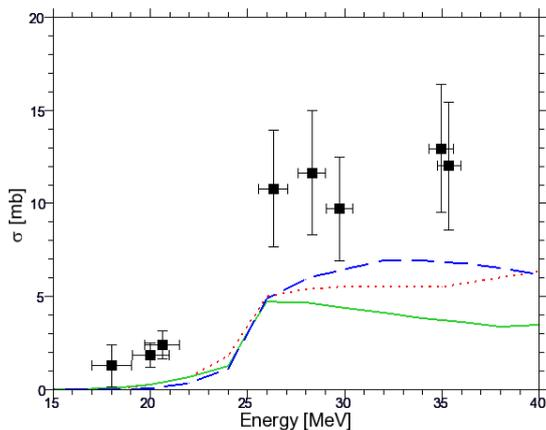
**Fig. 7.** Excitation functions for the  $^{12}\text{C}(^3\text{He}, \alpha+n)^{10}\text{C}$  reaction. ■: our data. Dotted line: TENDL-09 data base calculated with TALYS using default parameters. Solid line: ground state and first excited state calculated with TALYS and default parameters. Long dashed line: ground state with increasing the number of discrete levels considered with Hauser-Feshbach decay.
