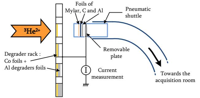
**Fig. 1.** Schematic view of the irradiation station.
