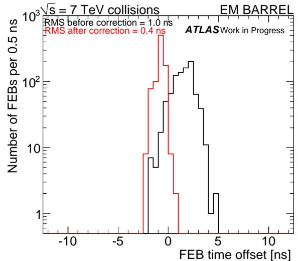
FIGURE 1.5 – For EM Barrel : the black histogram shows the FEB time offsets before the correction, and the red histogram shows the same distribution after the correction were applied.
