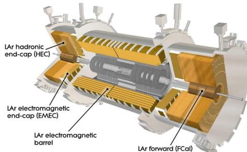
FIGURE 1.1 – Cut-away view of the ATLAS Liquid Argon calorimeter
