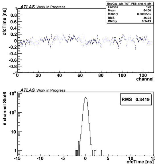
FIGURE 1.6 – For EM Endcap : in the upper plot on average the time versus the channel number in all the FEB in the middle layer with a  $\phi$  symmetry in the actual time situation ; in the bottom plot the channel time spread within a FEB in the middle layer, in the actual time situation.
