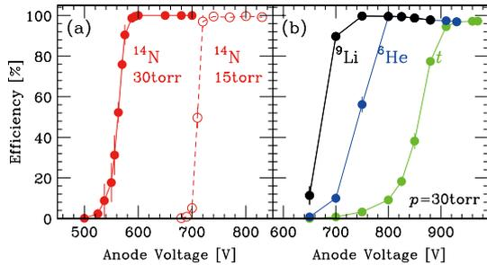
Fig. 3. (a) Detection efficiency for 250A-MeV  $^{14}\text{N}$  ions with the 15- and 30-torr operations. (b) Detection efficiency for  $t$ ,  $^6\text{He}$ ,  $^9\text{Li}$  particles with the 15- and 30-torr operations.
