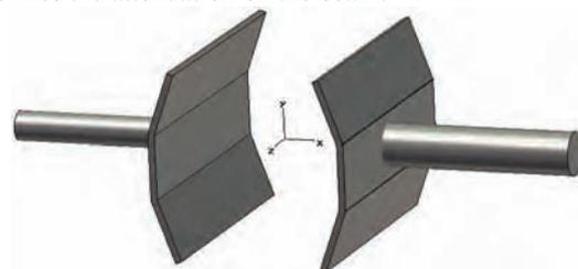
Figure 3: The electrode geometry; the plate bending angle is 20°.
