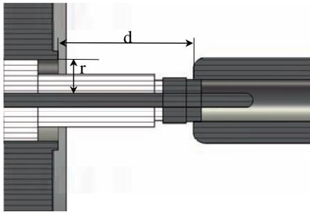
Figure 8: Section of the MDC-Cabum SHVE20-1-W feed-through.
