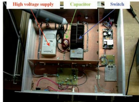
Figure 6: Scheme of the electronic cabinet.
