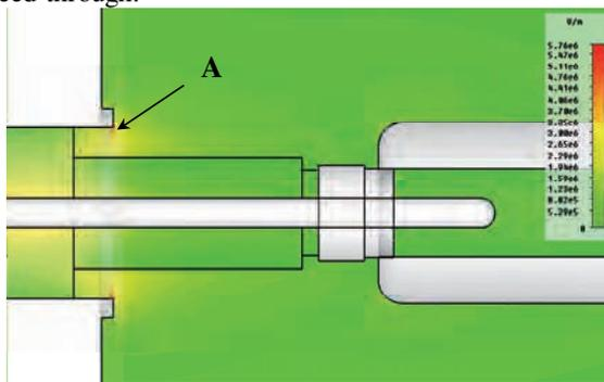
Figure 9: Electrostatic field on the section of the MDC-Cabum SHVE20-1-W feed-through.
