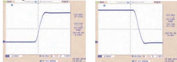
Figure 12: Measured rise and fall times.
