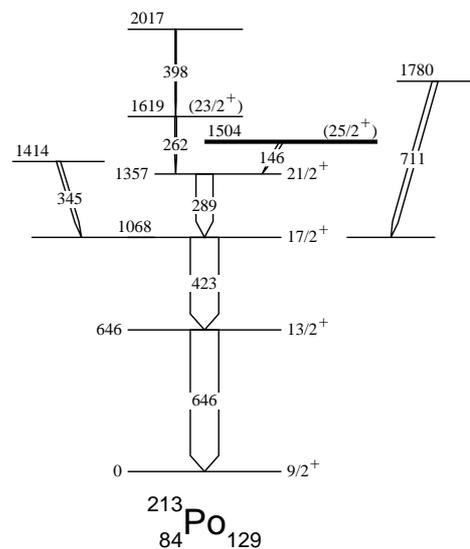
FIG. 2: Level scheme of  $^{213}\text{Po}$  determined in this work. The width of the arrows is representative of the relative intensity of the  $\gamma$ -rays. The level at 1504 keV is likely a long-lived state (see Sect. IV).
