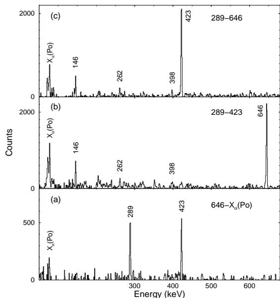
FIG. 1: Spectra of  $\gamma$ -rays in double coincidence with (a) the first transition of  $^{213}\text{Po}$  (646 keV) and the  $K_{\alpha 1}$  X-ray of Po, (b) the 289 keV and 423 keV transitions, and (c) the 289 keV and 646 keV transitions.
