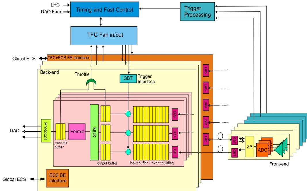
**Figure 1:** The readout scheme of the upgraded LHCb detector. The front-end is at the right and sends its data to the TELL40 boards which are the main pieces of the new DAQ design. The outputs of the TELL40 are copper cables connected to a large switch which dispatches the data to the event filter farm.
