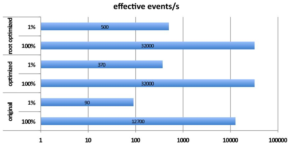
**Figure 5.** PROOF cluster reading full D<sup>3</sup>PD dataset from EOS. Shown are maximal sustained event rates.
