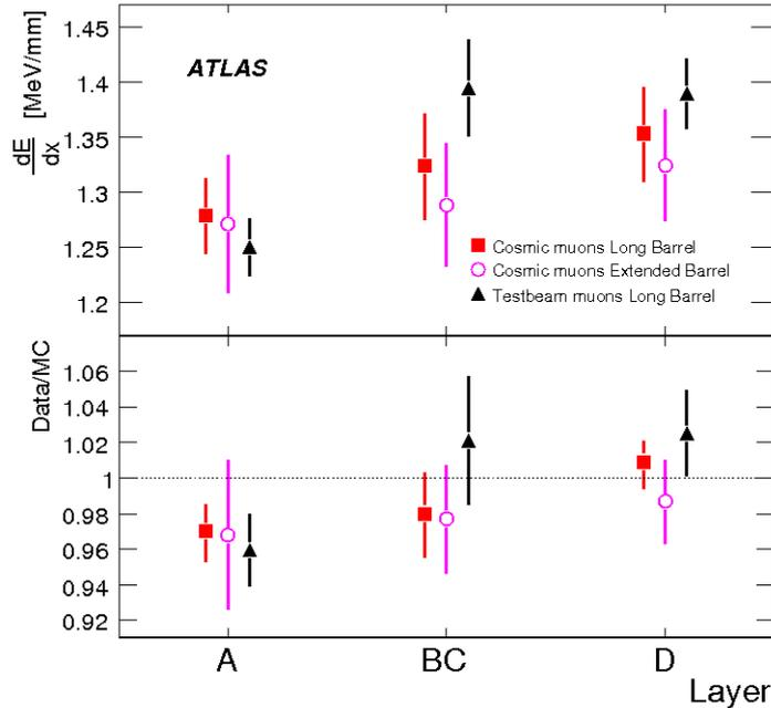
Figure 3: The truncated mean of the  $dE/dx$  for cosmic ray and testbeam muons shown per radial compartment and, at the bottom, compared to Monte Carlo. For the cosmic ray muon data, the results were obtained for modules at the bottom part of the calorimeter. The error bars shown combine in quadrature both the statistical and the systematic uncertainties, considering only the diagonal terms of the error matrix.
