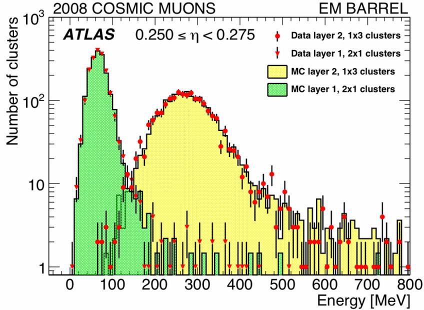
Figure 1: Energy in a  $2 \times 1$  cluster [10] in the first layer of the EM barrel (histogram for Monte Carlo and triangles for data) and in a  $1 \times 3$  cluster in the second layer (histogram for Monte Carlo and full circles for data) for all events
