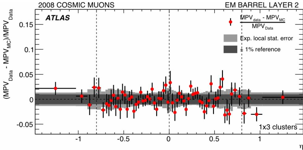
Figure 2: Measured  $U_{i,meas}$  (red points) and expected  $U_{exp}$  (light grey band) cosmic ray muon energy dispersions as function of  $\eta$  for the second layer of the EM barrel. The dark grey band indicates a  $\pm 1\%$  strip for reference.
