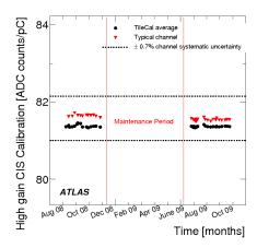
Figure 1. Time stability (1 year) of the average high gain CIS readout calibration constants.
