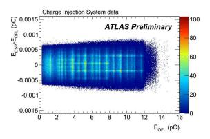
Figure 4. Absolute difference between the amplitude reconstructed online (DSP) and offline as a function of amplitude for CIS data in high gain.
