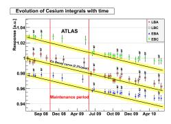
Figure 3. Evolution of TileCal response to radioactive Cesium source as a function of time.
