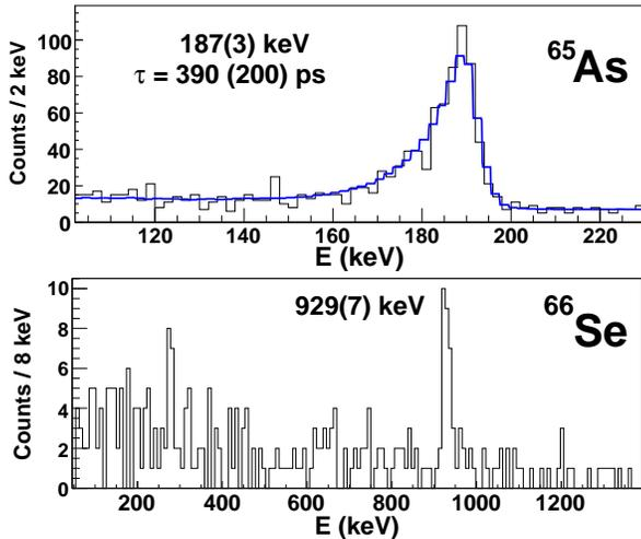
Figure 2: Doppler-effect corrected  $\gamma$  spectra of  $^{65}\text{As}$  (top) and  $^{66}\text{Se}$  (bottom). In the case of  $^{65}\text{As}$ , the best-fit simulated line shape (blue line) that corresponds to a lifetime  $\tau=390$  ps is superimposed to the experimental spectrum.
