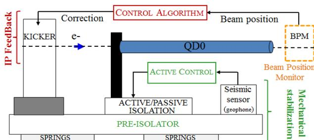
Figure 1: Overall layout of the FF stabilization.
