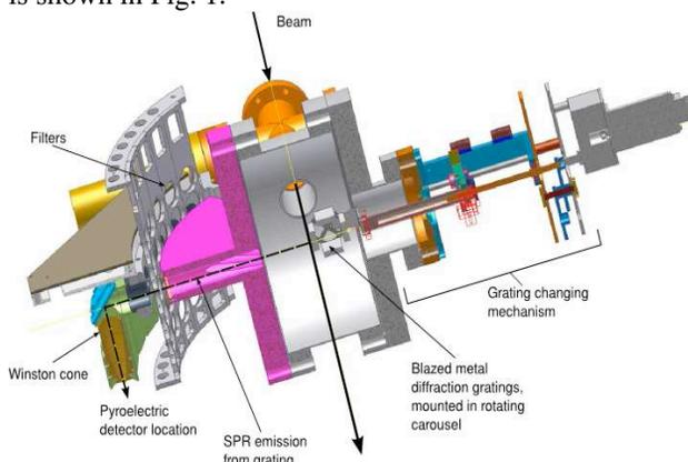
Figure 1: Layout of the Smith-Purcell vacuum chamber.
