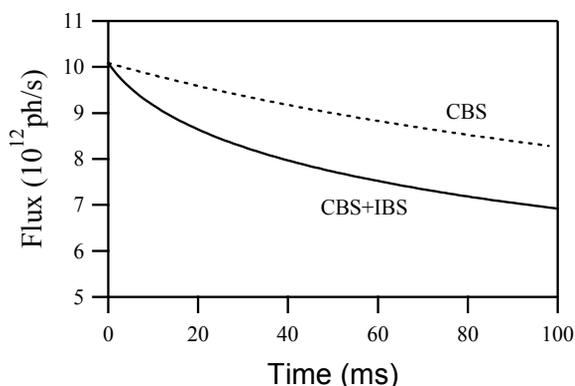
Figure 3: Total flux evaluated with eq. 3 versus time. Solid line: IBS and CBS are taken into account, dotted line: only CBS. Laser pulse energy : 30 mJ @ 1.06  $\mu\text{m}$ , Electron bunch charge 1 nC @ 50 MeV, IP transverse beam rms dimension 70  $\mu\text{m}$  ( $5 \cdot 10^{-8}$  of emittance), IP transverse laser pulse rms dimension 40  $\mu\text{m}$ , Laser pulse rms duration 20 ps, Electron beam rms duration 14 ps, Initial rms energy spread 0.3 %
