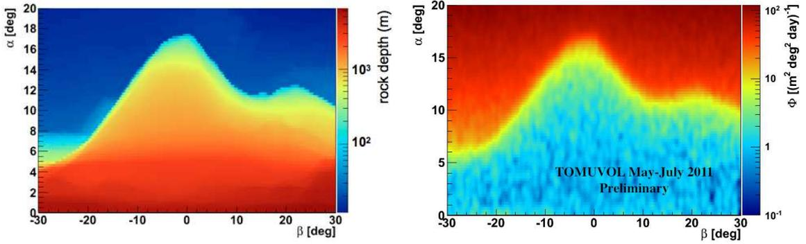
**Figure 1:** *Left:* Integrated path length that the atmospheric muons would have to travel through the volcano in order to reach the detector. *Right:* Shadow cast in the atmospheric muon flux by the Puy de Dôme, as measured with the second setup ( $\mathcal{A} = 1 \text{ m}^2$ , 1 m long).
