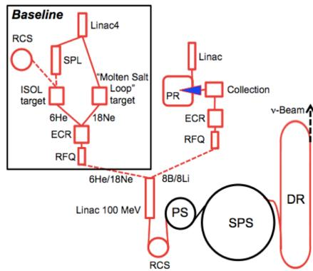
Figure 1: Layout of the CERN Beta Beam. Two beta emitting isotope pairs are considered:  ${}^6\text{He}/{}^{18}\text{Ne}$  (low-Q) with neutrinos to Fréjus and  ${}^8\text{Li}/{}^8\text{B}$  (high-Q) to Gran Sasso or Canfranc.
