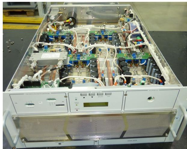
Figure 2: 7 kW amplifier unit.
