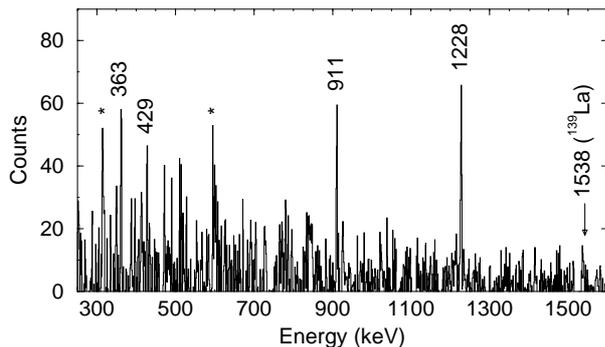
FIG. 1. Spectrum of  $\gamma$ -rays in double coincidence with the 1543- and the 323-keV transitions belonging to the yrast cascade of  $^{83}\text{As}$ . The weak 1538-keV transition is emitted by its main complementary fragment,  $^{139}\text{La}$ . The two lines marked with a star are identified contaminants.
