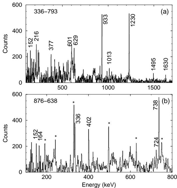
FIG. 3. Spectra of  $\gamma$ -rays in coincidence with two transitions of  $^{81}\text{As}$ : (a) with the 336- and the 793-keV transitions, (b) with the 876- and the 638-keV transitions. The lines marked with a star are identified contaminants.
