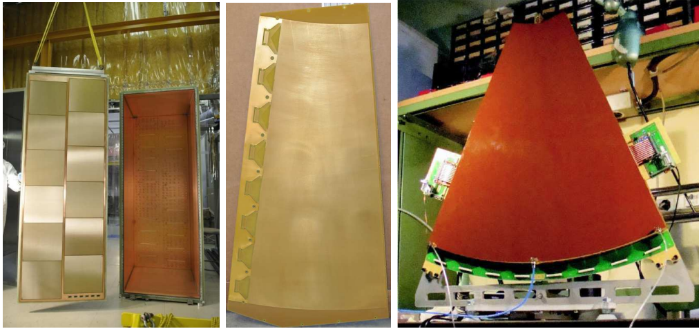
Figure 2. From left to right: photograph of a TPC for T2K showing an endplate ( 0.7\times 2\text{ m}^2 ) with Micromegas modules and the field cage; 1 m long Bulk mesh with strip readout for Super ATLAS; triple GEM chamber for the TOTEM tracking system ( 0.2\text{ m}^2 ).
