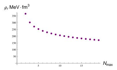
Fig. 16. The values of g that reproduce the observed  $0^+-2^+$  energy splitting in  ${}^6\text{He}$  as a function of the number of shells in the valence space.
