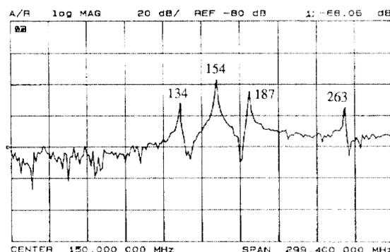
Fig. 4 : Frequency spectrum measured on the half-scale model for the 430 MeV/n cyclotron cavity (fourth harmonic).
