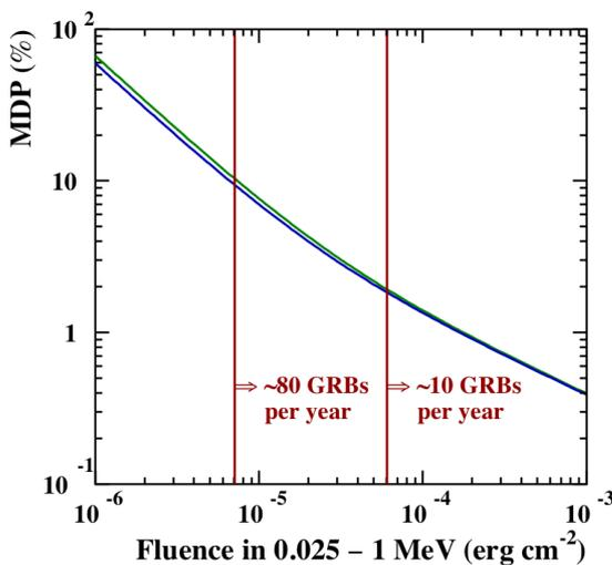
**Figure 3-2:** Minimum polarization detectable by CAPSiTT in the range 0.2 – 2 MeV as a function of the GRB fluence. The assumed GRB duration is 50 s and the source spectrum is a Band law with  $\alpha = -1.1$ ,  $\beta = -2.3$  and  $E_{\text{peak}} = 200 \text{ keV}$  (green curve) or 1 MeV (blue curve).
