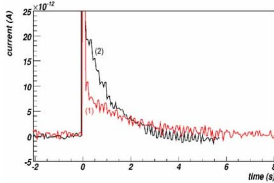
Fig. 2. Current transients at  $T = 410$  mK for two different detector biases, showing the field effect on carrier emission. Transients (1) and (2) correspond to field intensities of 1.8 V/cm and 11 V/cm respectively (see text).
