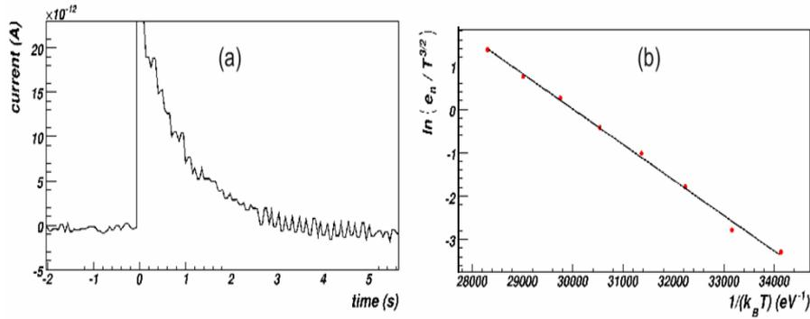
Fig. 1. (a) Current emission transient under 24 V detector bias (see text). The overshoot of the signal at  $t = 0$  is an artifact of the measurement. (b) Arrhenius plot of the emission rate as a function of  $1/k_B T$ , giving the activation energy for carrier emission from the trap as  $E_t = (0.75 \pm 0.02)$  meV.
