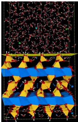
**Fig. 1.** The interfacial fragment of the MD simulation cell. The tobermorite structure is represented by distorted Ca-octahedra (blue), Si-tetrahedra (yellow), O (red balls), H (white balls). Water molecules are shown as red and white sticks, while the green and light blue balls represent Cl<sup>-</sup> and K<sup>+</sup> ions, respectively.
