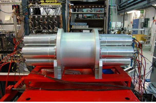
Fig. 1. (Color online) View of the total absorption spectrometer without lead shielding.
