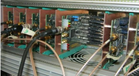
Figure 6: zoom on the 16-channel WaveCatcher crate
