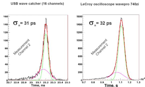
Figure 9: WaveCatcher module vs LeCroy oscilloscope
