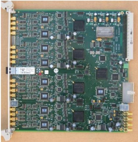
Figure 10: the 16-channel WaveCatcher board
