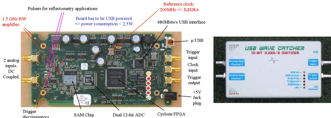
Figure 2 & 3: the USB-powered USB\_WaveCatcher board (3.2GS/s, 12 bits, time resolution < 10ps rms)
