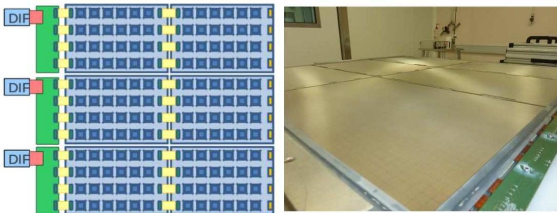
**Figure 1.** Drawing and photograph of the ASIC and mesh sides of the 1 m<sup>2</sup> chamber.
