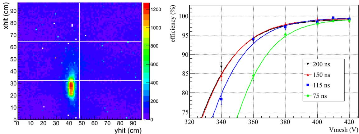
**Figure 2.** Profile of a muon beam crossing the 1 m<sup>2</sup> chamber before applying a cut on the trigger time (left). Efficiency versus mesh voltage curves for various peaking times (right).
