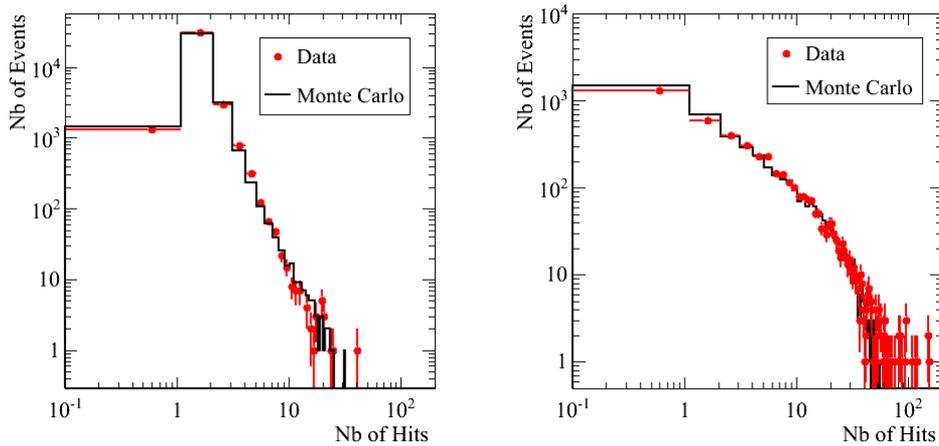
**Figure 4.** Hit distribution from 100 GeV muons (left) and pions (right) as measured at layer 48 of a hadron calorimeter (setup (ii)). Data points are compared to Monte Carlo predictions from GEANT4 LHEP physics list. The mesh voltage was 390 V during both runs.
