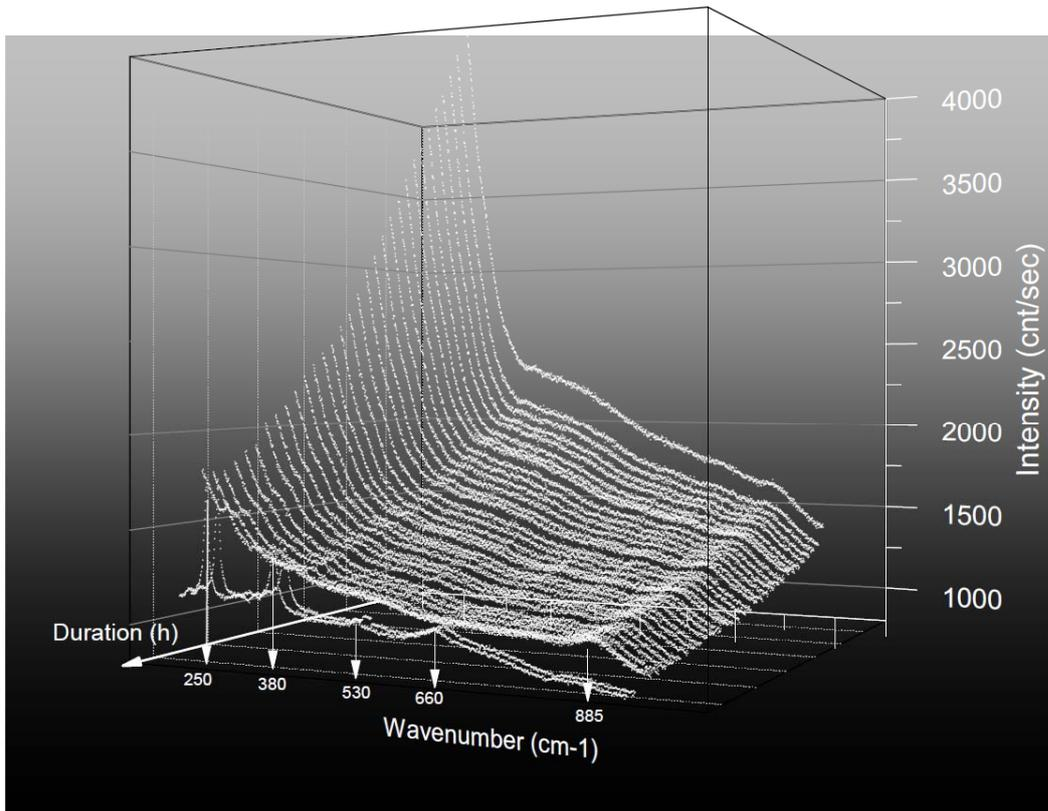
Figure 4: Raman spectra of set IV during the *in situ* experiment with an experimental time of 15 h after the irradiation. Corroded carbon steel sample with formation vs. time of the typical Raman bands of lepidocrocite phase at 250/380/530/660  $\text{cm}^{-1}$  and  $\text{H}_2\text{O}_2$  Raman band at 885  $\text{cm}^{-1}$
