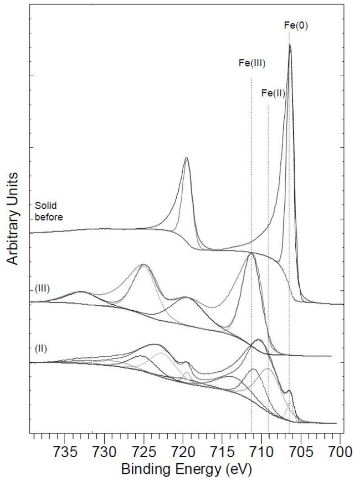
Figure 3: Fe<sub>2</sub>p XPS spectra obtained onto the two solid samples before irradiation but after the etching process with Fe(0) component, the iron sample (set II) with the Fe(II)/Fe(III) components and the carbon steel sample (set III) with the Fe(III) component (cf. Table 3)
