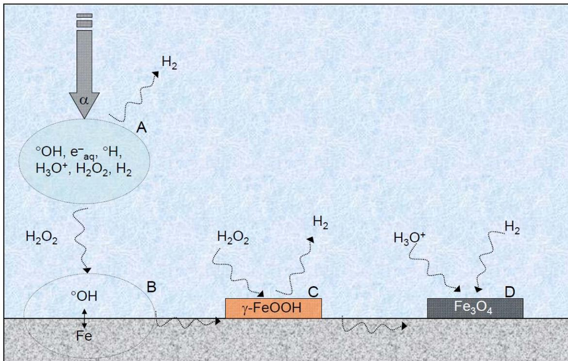
Figure 5: Scheme of iron corrosion mechanisms under  ${}^4\text{He}^{2+}$  ions irradiation, (A) water radiolysis, (B)  $\text{H}_2\text{O}_2$  catalytic decomposition and iron oxidation, (C) Lepidocrocite  $\gamma\text{-FeOOH}$  formation with  $\text{H}_2$  production (carbon steel sample), (D) Magnetite  $\text{Fe}_3\text{O}_4$  formation with  $\text{H}_2$  consumption (pure iron sample)
