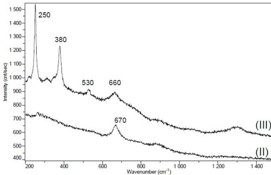
Figure 2: Corroded iron sample (set II) with Raman band of magnetite phase at  $670 \text{ cm}^{-1}$  and corroded carbon steel sample (set III) with Raman bands of lepidocrocite phase at  $250/380/530/660 \text{ cm}^{-1}$  identified in the literature [48]
