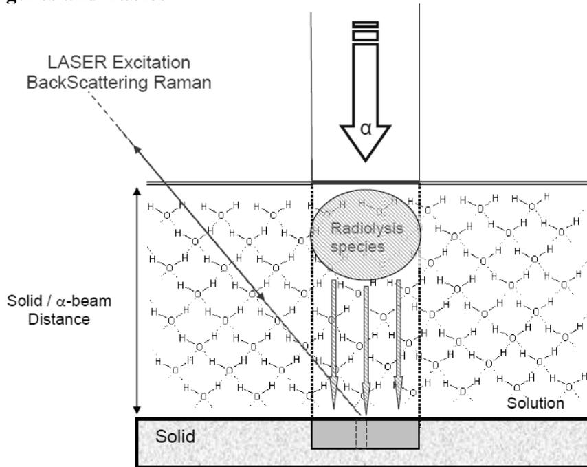
Figure 1: *In situ* Raman spectroscopic device experiment under  $^4\text{He}^{2+}$  ions beam irradiation onto the ARRONAX facility vertical beam line (Borosilicate Glass Disc Thickness =  $150 \pm 10 \mu\text{m}$ , Electrolyte Thickness = 5 mm)
