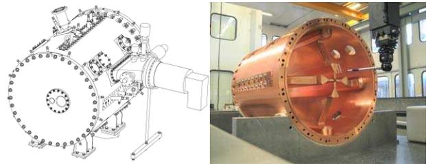
Figure 3 : SPIRAL 2 RFQ prototype cavity
