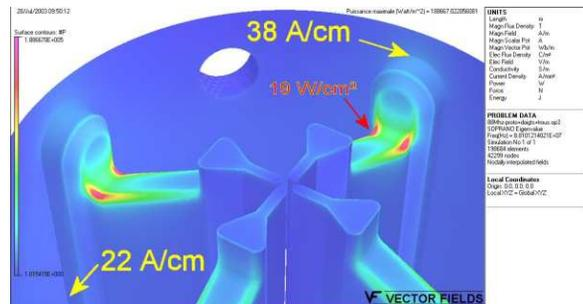
Figure 4: 3D view of the power deposition
