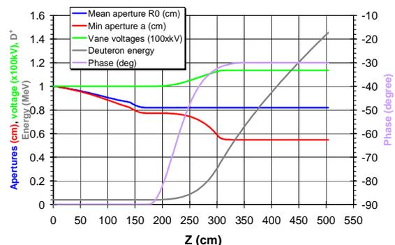
Figure 2 : Main parameters of the RFQ
