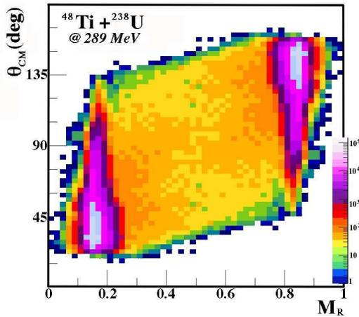
Figure 1: Correlation between the center-of-mass deflection angle ( $\theta_{CM}$ ) and the mass ratio ( $M_R$ ).
