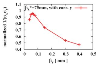
Figure 7: The geometric luminosity normalized by the original one ( $\beta_x^*/\beta_y^*=15\text{mm}/0.4\text{mm}$ , correction in both plane) as a function of  $\beta_y^*$  when  $\beta_x^*=75\text{mm}$ .
