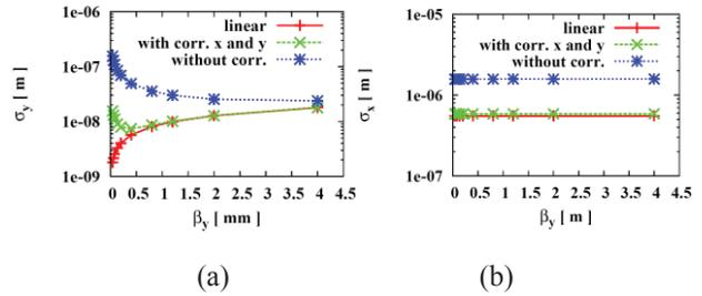
Figure 4: (a) The vertical beam size  $\sigma_y^*$  as a function of  $\beta_y^*$  when  $\beta_x^*=15\text{mm}$ . (b) The impact of the variable  $\beta_y^*$  on  $\sigma_x^*$  when  $\beta_x^*=15\text{mm}$ .
