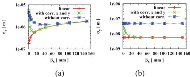
Figure 3: (a) The horizontal beam size  $\sigma_x^*$  as a function of  $\beta_x^*$  when  $\beta_y^*=0.4\text{mm}$ . (b) The impact of the variable  $\beta_x^*$  on  $\sigma_y^*$  when  $\beta_y^*=0.4\text{mm}$ .
