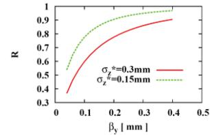
Figure 8: Analytic luminosity reduction due to hour-glass effect.
