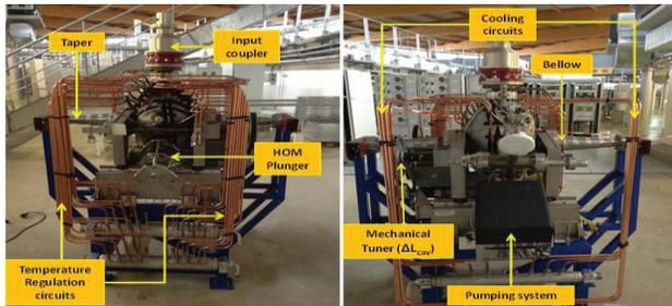
Figure 1: ThomX cavity assembly (front and back views).
