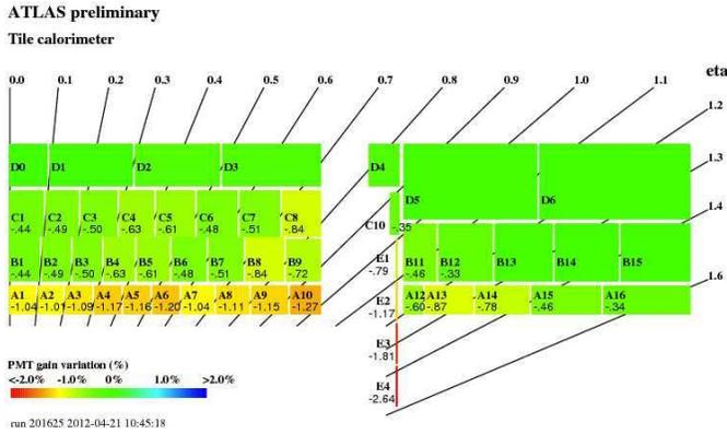
Fig. 5. Mean gain variation (in %) in the PMTs of the Tile Calorimeter, between the 19<sup>th</sup> March 2012 and the 21<sup>st</sup> April 2012 (between 2 consecutive Cesium scans)
