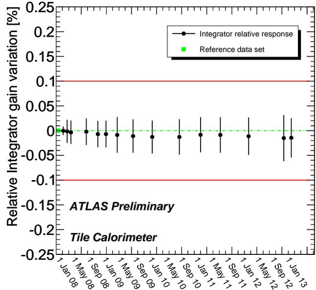
Fig. 7. Relative variation of the integrator gain used by the Cesium calibration system obtained by comparing the gains of all the channels of the Tile Calorimeter
