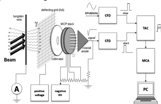
Figure 1: Principal schema of operation of BEM electronics.
