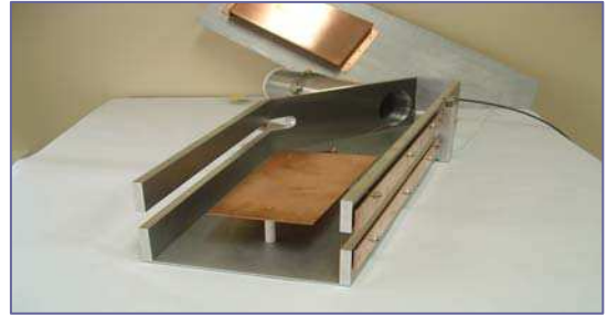
Figure 3: View of the prototype device with the upper part and electrode lifted off.
