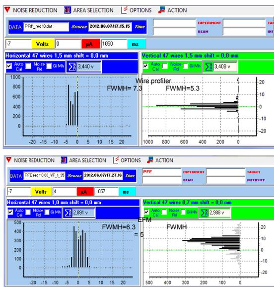
Figure 8: Profile comparison between grid profiler and EFM.
