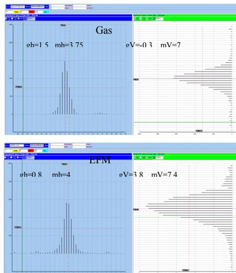
Figure 6: Obtained profiles on the two profilers with 10<sup>6</sup> pps of <sup>40</sup>Ar<sup>6+</sup> beam: gH and gV are the centroid position of the profile with respect to the central position of the beam and mH or mV are the FWHM of each profile.
