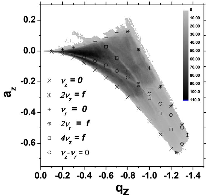
Figure 5: The first stability domain of the LPCTrap as obtained by the simulations for  $Ca^+$  ions. The symbols give the theoretical limits of the domain and the positions of the non linear resonances.
