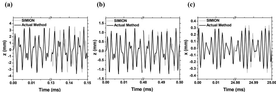
Figure 3: Evolution of the position of an ion starting from the origin with different initial kinetic energies  $E_0$ . Working point ( $q_z = -1.32, a_z = -0.54$ ) (a)  $E_0 = 0.1$  eV with the motion in the  $z$ -direction. (b)  $E_0 = 0.01$  eV with the motion in the  $z$ -direction. (c)  $E_0 = 0.1$  eV with the motion in the  $x$ -direction.
