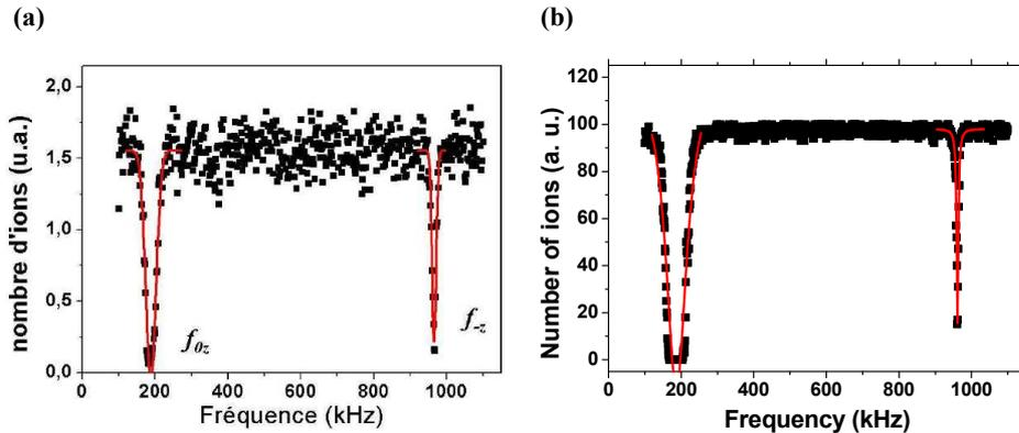
Figure 9: (a) Experimental dipole excitation spectrum of  ${}^6\text{Li}^+$  for  $V_{AC} = 60\text{ V}$  and  $f = 1.15\text{ MHz}$  obtained from Ref. [16]. (b) The simulated spectrum for the same conditions
