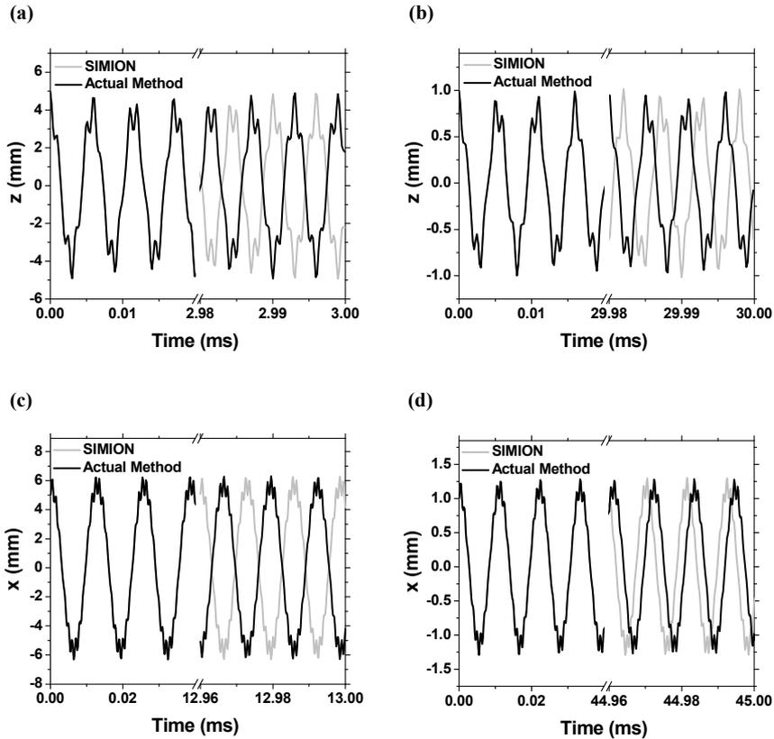
Figure 2: Evolution of the position of an ion starting from rest at different initial positions  $(x_0, y_0, z_0)$ . Working point  $(q_z = -0.5, a_z = 0)$  (a)  $x_0 = y_0 = 0, z_0 = 5 \text{ mm}$ . (b)  $x_0 = y_0 = 0, z_0 = 1 \text{ mm}$ . (c)  $x_0 = 5 \text{ mm}, y_0 = z_0 = 0$ . (d)  $x_0 = 1 \text{ mm}, y_0 = z_0 = 0$ .
