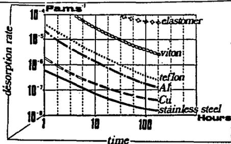
Fig. 7 : Desorption rate of various materials.
