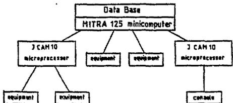
Fig. 1 : Logical structure of the control system.
