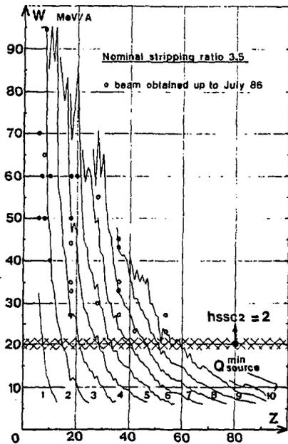
Fig.5. Energies computed (solid lines) and obtained (dots) as a function of the charge state of the PIC or ECR source. Stripping ratio 3.5.
