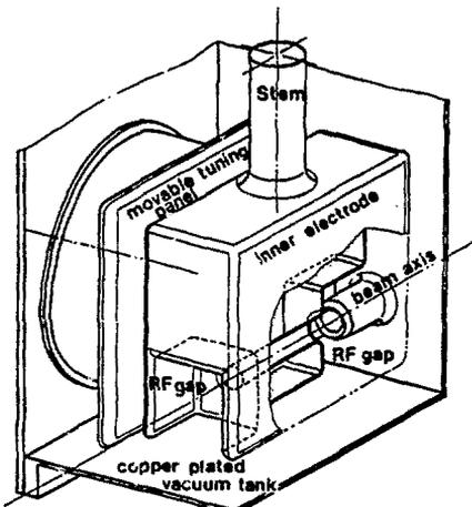
Fig.6. A view of buncher R1 with the modified RF gaps.
