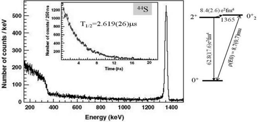
Figure 1. Electron Energy Spectrum showing the  $0^+_{2}-0^+_{1}$  E0 transition in  $^{44}\text{S}$  Left the low excitation energy spectrum of  $^{44}\text{S}$  [6]
