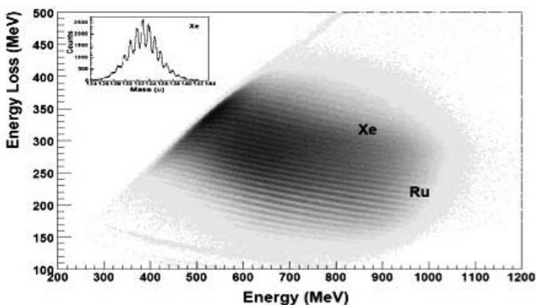
Figure 3 : Two dimensional spectrum of  $\Delta E$  vs.  $E_{\text{total}}$  in the  $^{238}\text{U}+^{12}\text{C}$  system at an incident beam energy of 1.45 GeV. The inset shows the associated mass spectrum for the Xe isotopes.
