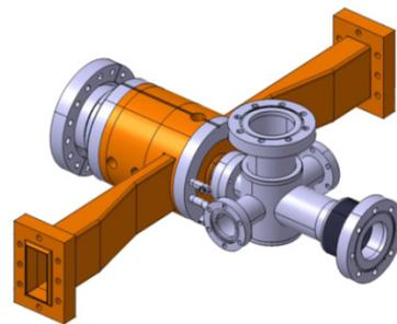
Figure 3: Drawing of the 2998MHz ThomX electron gun.
