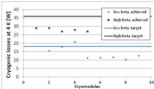
Figure 4: Total cryogenic losses of cryomodules at 4 K.
