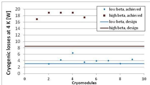
Figure 5: Static cryogenic losses of cryomodules at 4 K.
