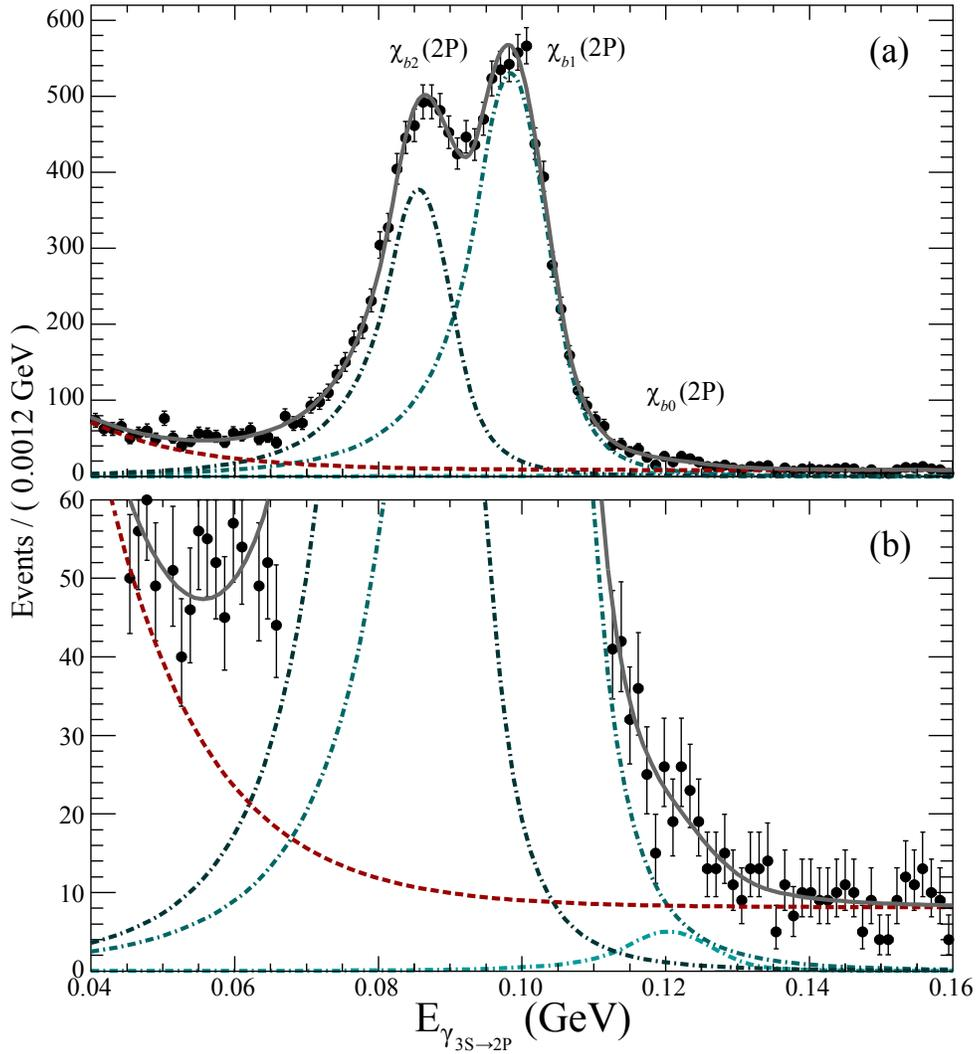
FIG. 5: (a) Fit to the soft photon energy  $E_{3S \rightarrow 2P}$  in the  $3S \rightarrow 2P \rightarrow 1S$  cascade with individual signal (signal corresponds to the small bump) and background (dash) components for the calorimeter-based analysis. (b) A zoomed-in view of the  $\chi_{b_0}(2P)$  peak on the same energy scale. Discussion of the significance of the  $J = 0$  peak is contained in Section IV C.
