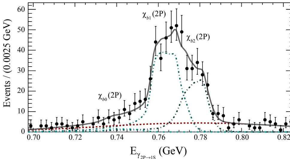
FIG. 9: Fit to the photon energy  $E_{2P \rightarrow 1S}$  in the  $3S \rightarrow 2P \rightarrow 1S$  cascade for the conversion analysis. The data are represented by points, the total fit by a solid curve, the background component with a dotted curve, and the individual signal components of the fit by peaking dot-dashed curves in progressively darker shades for  $J = 0, 1, 2$ . Clear signals for the  $J = 2$  and  $J = 1$  signals are seen.
