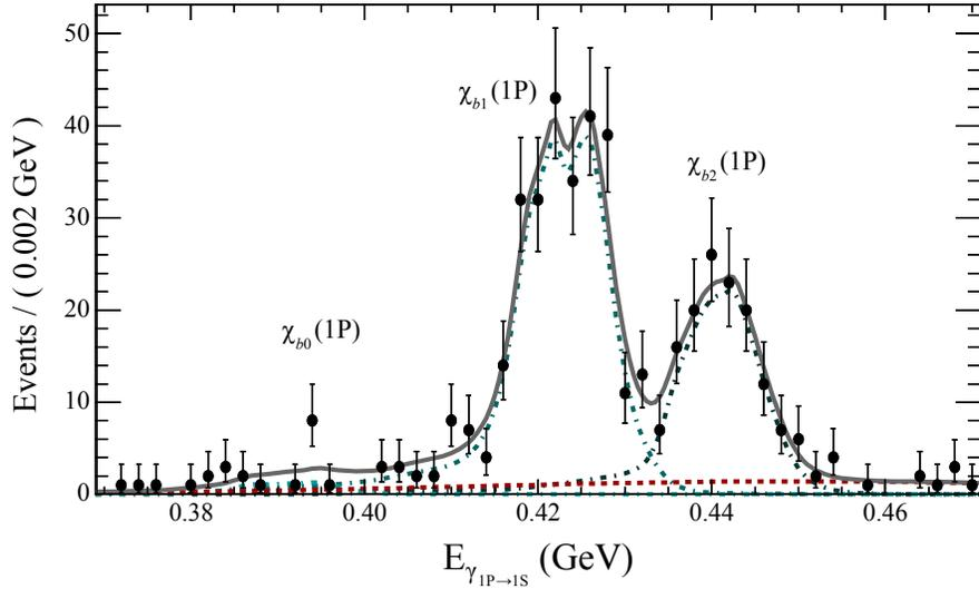
FIG. 6: Fit to the photon energy  $E_{1P \rightarrow 1S}$  in the  $2S \rightarrow 1P \rightarrow 1S$  cascade for the conversions analysis. The data are represented by points, the total fit by a solid curve, the background component with a dashed curve, and the individual signal components of the fit by peaking dot-dashed curves in progressively darker shades for  $J = 0, 1, 2$ . Clear evidence is seen for the  $J = 2$  and  $J = 1$  signals.
