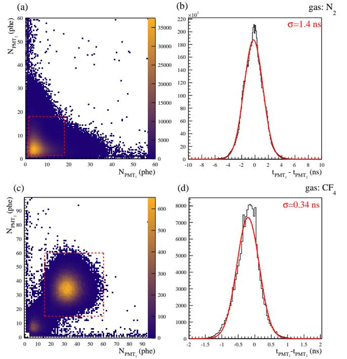
FIG. 7: (a) Correlation plot and (b) time coincidence distribution for  $N_2$ , and (c), correlation plot and (d) coincidence time spectrum for  $CF_4$ . The red dashed lines indicate the selections made for building the coincidence time spectra, the red solid lines represent the Gaussian fits applied to extract the coincidence time resolutions.
