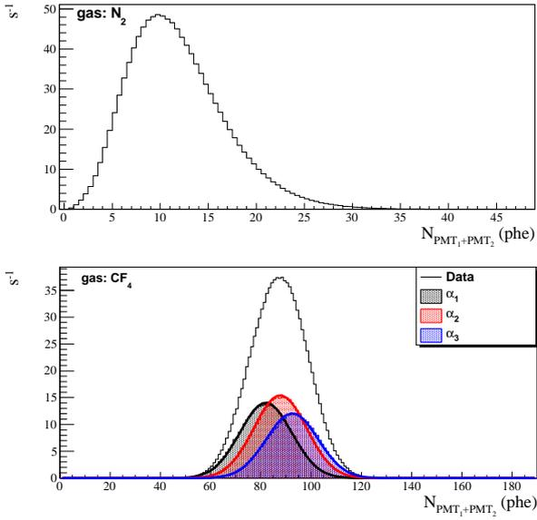
FIG. 6: (top) Sum of the photoelectrons seen by the PMTs for  $N_2$ . (bottom) Sum of the photoelectrons seen by the PMTs for each  $\alpha$  energy selected by the IC and fitted by a Gaussian distribution for  $CF_4$ .
