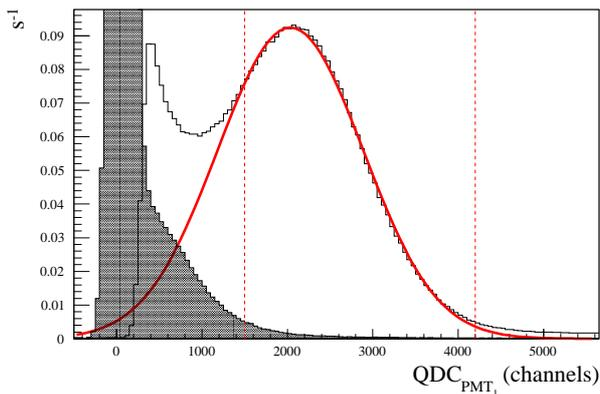
FIG. 2: SPE calibration spectrum for PMT<sub>1</sub>, QDC<sub>1</sub> is plotted unfilled and QDC<sub>2</sub> is black filled. The solid red line correspond to the Gaussian fit of one photoelectron. The vertical dashed lines show the fit intervals.
