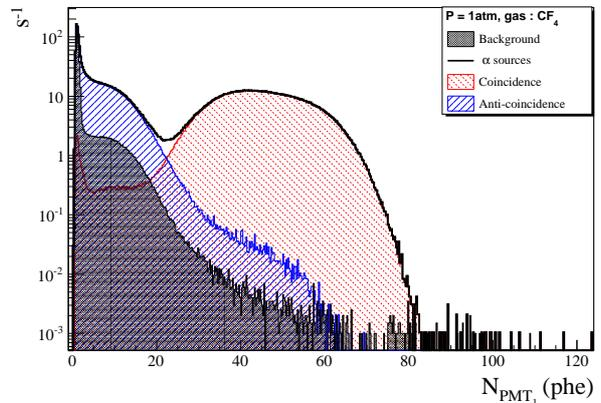
FIG. 3: Distribution of photoelectrons in one PMT induced by  $\alpha$  particles (black line histogram) for CF<sub>4</sub> at atmospheric pressure, the dashed line filled (red) histogram corresponds to coincidence between the two PMTs and the filled with solid lines (blue) histogram corresponds to anti-coincidence. The dot filled (black) histogram corresponds to background acquisition.
