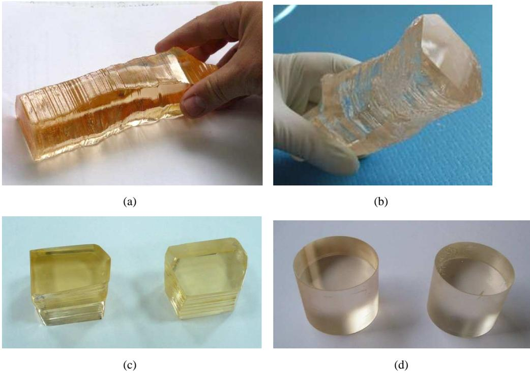
**Figure 1.** Large volume zinc molybdate crystal boules with mass  $\sim 1$  kg developed as a precursor (a) and in the framework of the LUMINEU program (b) (see text). Scintillation elements with mass of about 0.3 kg produced from precursor (c) and LUMINEU (d)  $\text{ZnMoO}_4$  crystal boules.
