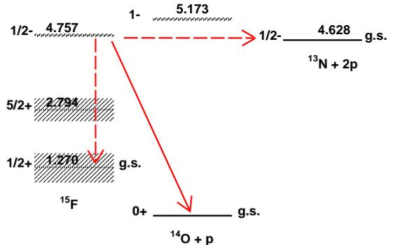
Figure 2: (Color online) Level scheme of  $^{15}\text{F}$ . The possible decay channels from the  $J^\pi=1/2_1^-$  resonance are: the one proton emission (red arrow), gamma transition and two proton emission (red dashed arrow). The hatched areas correspond to the width of the resonances.
