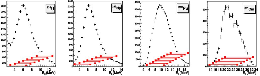
**Figure 1.** Distribution on excitation energy for each fissioning system produced by transfer reactions. Red lines indicates the gates on excitation energy considered for investigate the evolution of the fission-fragment distribution with the excitation energy.
