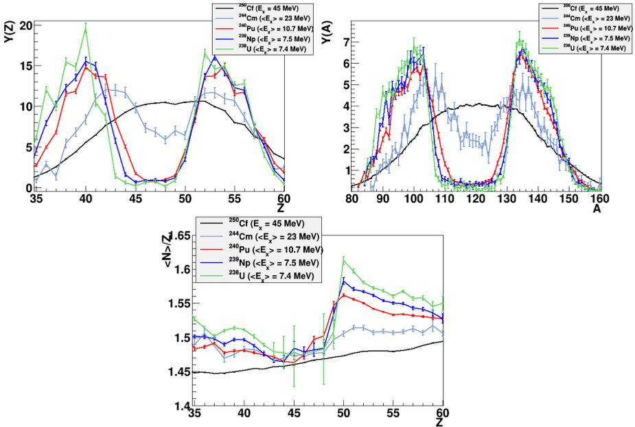
**Figure 2.** (a) Atomic number distributions of fission fragments for different fissioning systems. (b) Mass distributions of post-neutron evaporation fission fragments. (c) Neutron excess of post-neutron evaporation fission fragments as a function of their atomic number.
